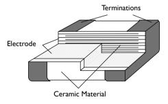
Surface mount multilayer ceramic capacitor construction
