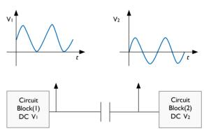
Coupling capacitor separates DC voltages of circuit blocks but couples AC signal.
