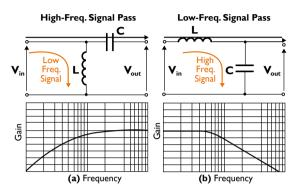
Filtering functions of capacitor coupled with inductor
